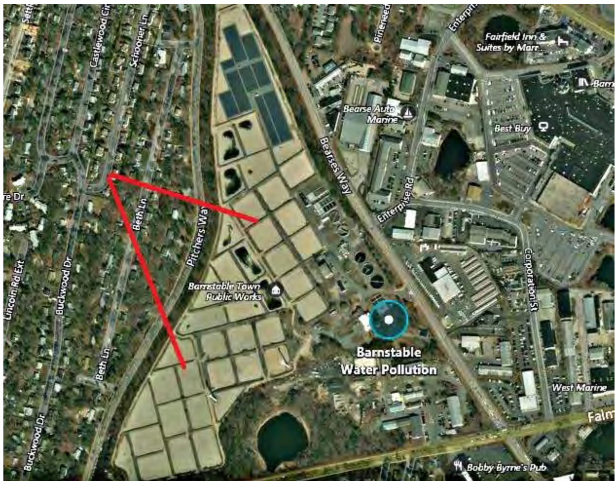
Water Pollution Control Sand Filter Beds
