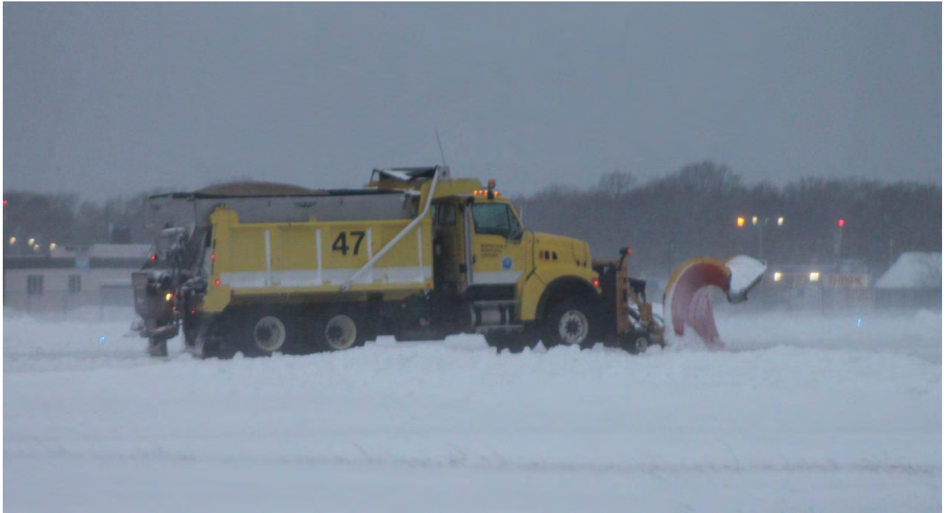
2006 Sterling A Line Diesel Heavy Duty Carrier Vehicle with Plow and Sander
